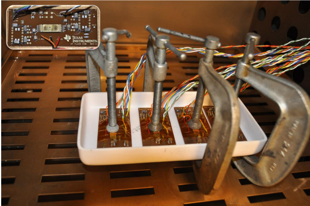
Figure 1. Technique for securing the flash modules in the oven. (Inlay) Modified flash module with HMP solder, high temperature ceramic capacitors and Teflon coated nickel wire.
